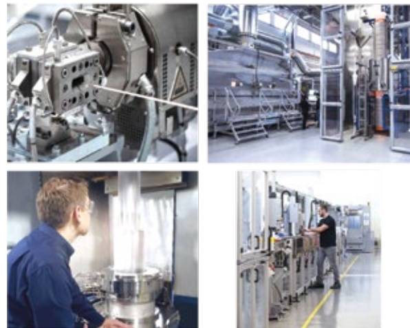
Clockwise from top left: Rosendahl's hairpin extrusion with a newly developed flat crosshead, Nextrom's preform lab in Vantaa, Nextrom's induction furnace for optical fiber preforms and Rosendahl's newly installed loose tube laboratory line in Pischelsdorf.
